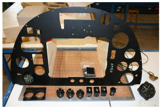
The dashboard with seven coats of matt black paint and the various switches and gauges we have been given.
