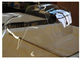
main canopy with correct flat-sides and pilot's knockout panel, and the rear canopy, essentially a glorified hoop of Perspex fixed between frames 11 and 12. The optical clarity of the workmanship that has gone in to making the glazing is stunning, and they really are a thing to behold. The company who produce them make the canopies for the Battle of Britain Memorial Flight aircraft, as well as racing car screens among other
